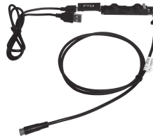
Illustration 1.2.2_2: Universal programming tool
