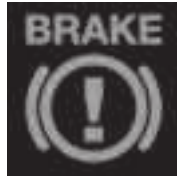
Illustration 6.5_2: Brake sensor active
